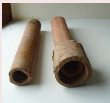
Clay land drains
